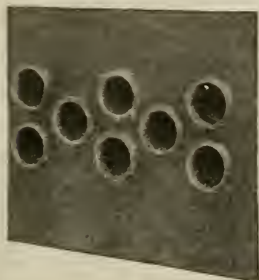
SECTION OF LOCOMOTIVE FLUE SHEET WITH TUBES IN PLACE READY FOR WELDING.
